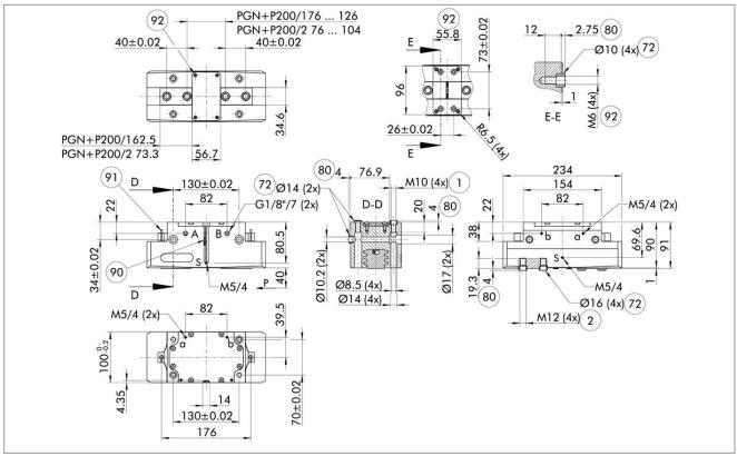
The drawing shows the gripper in the basic version with closed jaws, without dimensional consideration of the options described below.
