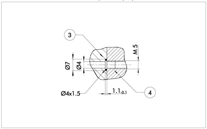
The direct connection is used for supplying compressed air without hoses. Instead, the pressure medium is fed through bore-holes in the mounting plate.
