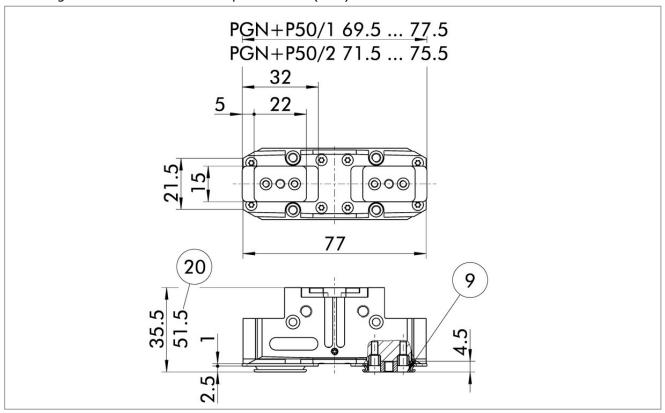
The dust cover option increases the protection against external particles. The assembly diagram shifts by the height of the intermediate jaw. The finger length is still measured from the upper edge of the gripper housing.
