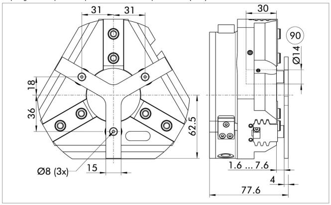
For spring-supported positioning of the workpiece against a stop after the gripper has opened. Especially developed for loading machines.
