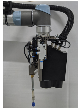
Fig. 1 - Energy Chain with 0 degrees rotation of the 6th axis.
