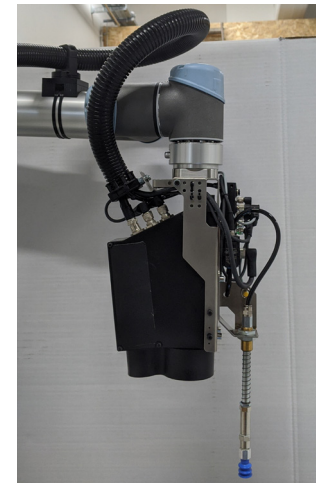
Fig. 2 - Energy Chain with 180 degrees rotation of the 6th axis.
