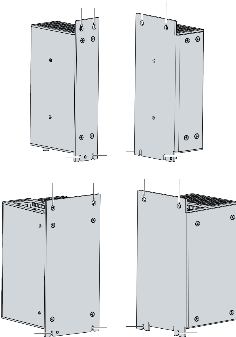
Fig. 21: C6920_Dismantling the control cabinet
