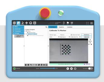
"Calibrate to Marker" functionality provided as UR program nodes for a seamless integration into programs and fast runtime calibration between robot and markers.
