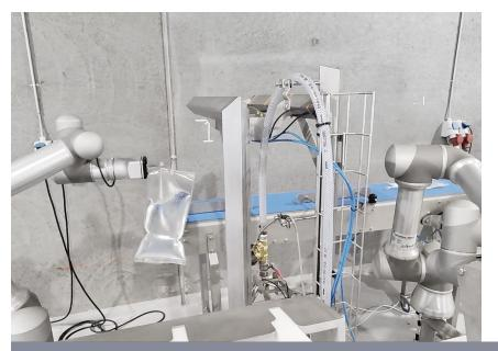
For a large Danish food company, Technicon has developed a flexible automation solution consisting of two UR5e and cleanroom grippers from OnRobot and associated software.
